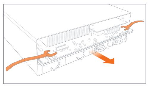
**Figure 19** Control Card Removal
