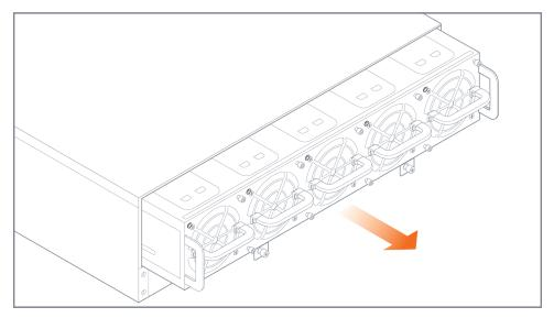
Figure 11 Fan Tray Removal
