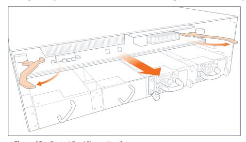
**Figure 18** Control Card Ejector Handles
