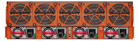
Figure 6 Four Power Supply Modules Installed
