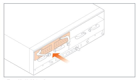
**Figure 11** *Module Insertion*
