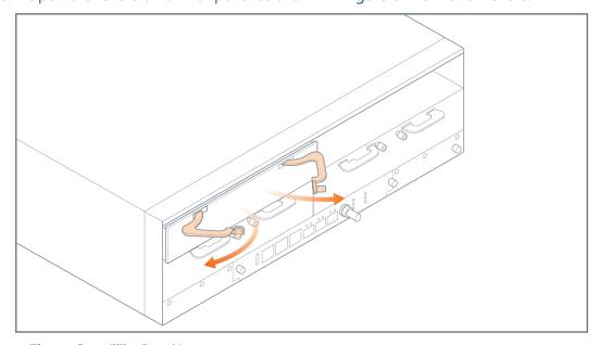
Figure 8 Filler Panel Levers
