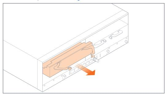
Figure 9 Filler Panel Removal
