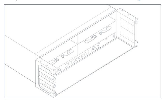
Figure 3-7: Cable Management Sides and Bottom Plate
