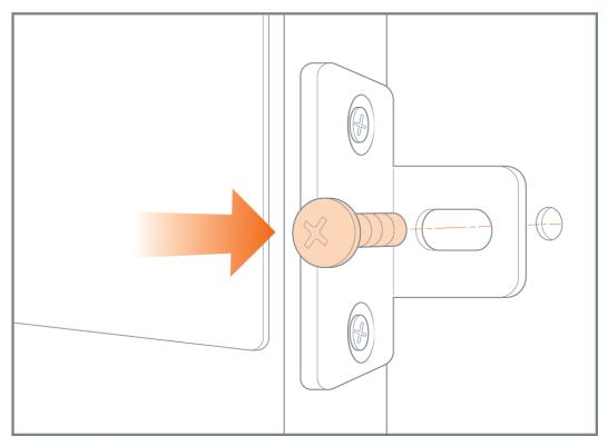
**Figure 4** Locking Rack Ear Attached to Rack
