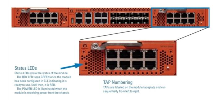
Figure 4 GigaVUE-HC3 Extension Board
