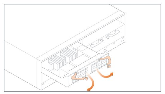
Figure 10 Module Levers
