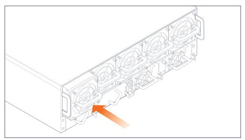
**Figure 14** Fan Module Insertion
