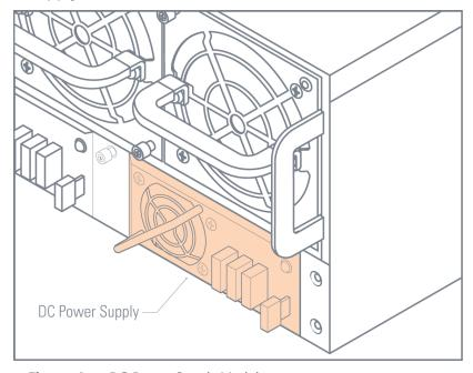
Figure 4 DC Power Supply Module
