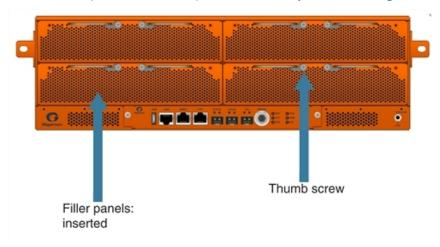
**Figure 7** Filler Panels Inserted
