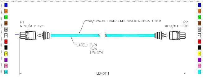
**Figure 1** MPO/MTP 12 Position Fiber Cable
