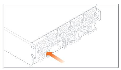
**Figure 9** Fan Module Insertion
