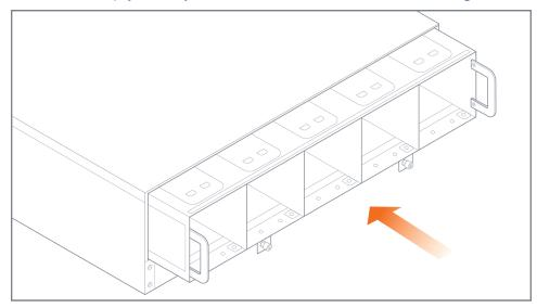
**Figure 12** Fan Tray Insertion
