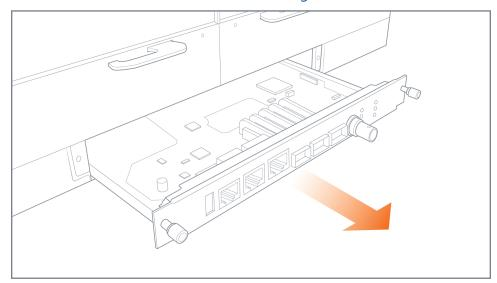
Figure 16 Extension Board Removal
