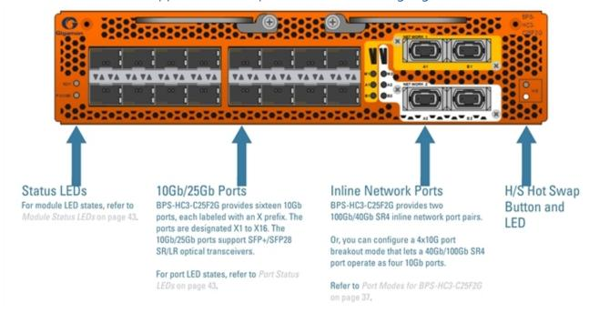
Figure 9 BPS-HC3-C25F2G Module
