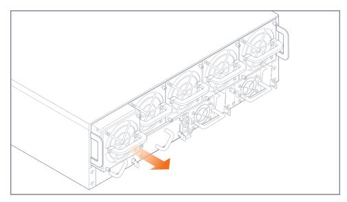
**Figure 8** Fan Module Removal
