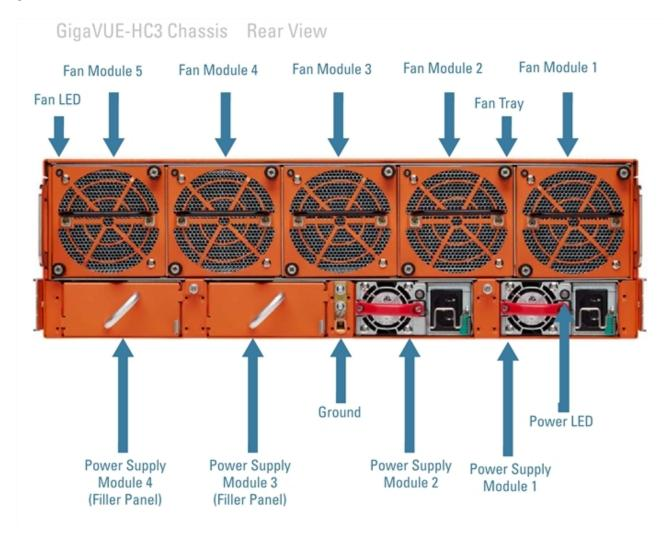
**Figure 3** Rear View of the GigaVUE-HC3 Chassis
