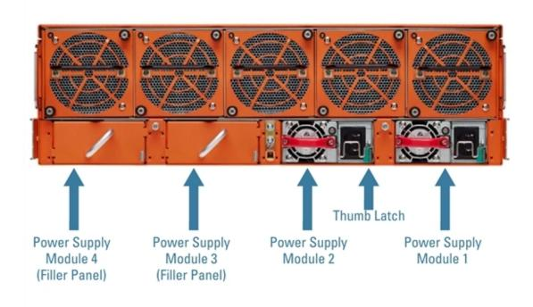
**Figure 5** Power Supply Modules (AC Version Shown)
