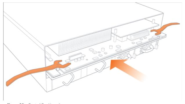
**Figure 20** Control Card Insertion
