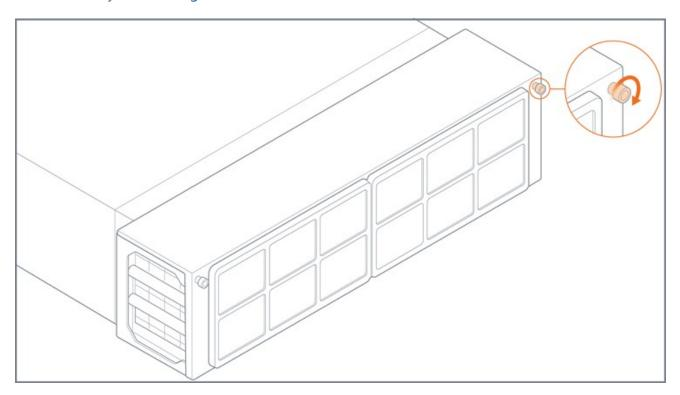
Figure 3-8: External Air Filter
