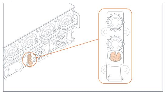
**Figure 1** Grounding Lug on Rear of GigaVUE-HC3
